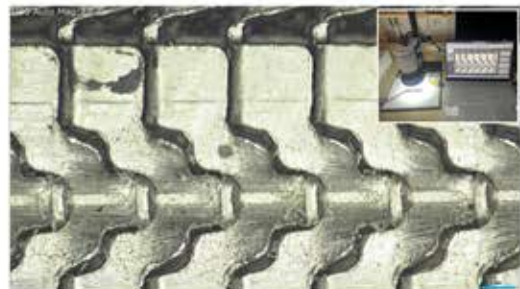
Rough machined heat sink
